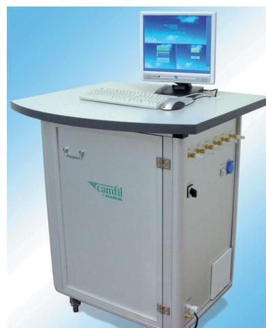
The CamContain Filter Validation System (FVS) is an integrated and intelligent auto-scanning software package that allows for validation tests to occur while labs are still active. Innovative in design, and configurable to meet proprietary requirements, the CamContain FVS increases the quality and accuracy of revalidation procedures by reducing exposure to test personnel and adjacent environments, while increasing the speed of in situ tests.
