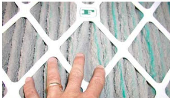
Filter Test: The 30/30 after only four months of operation.
