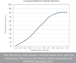
The Camfil Aeropleat IV extended surface pleated filter offers more media for high dirt-loading applications. The Aeropleat IV has a MERV 8 when evaluated per ASHRAE Standard 52.2.
